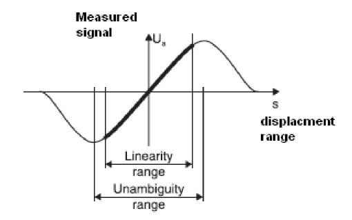
Linearity of the measurement signal of an inductive displacement sensor
