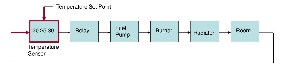
The block diagram represents the system components, the thermostat block process two input signals, a room temperature and a temperature set point to produce one output signal that is sent to a mechanical relay switch. The thermostat acts as a primary sensor and transducer.
