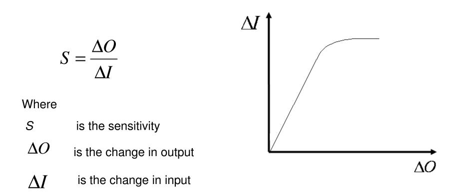
Example, if a movement of 0.001mm causes an output voltage change of 0.02V, the sensitivity of the measuring instrument is
