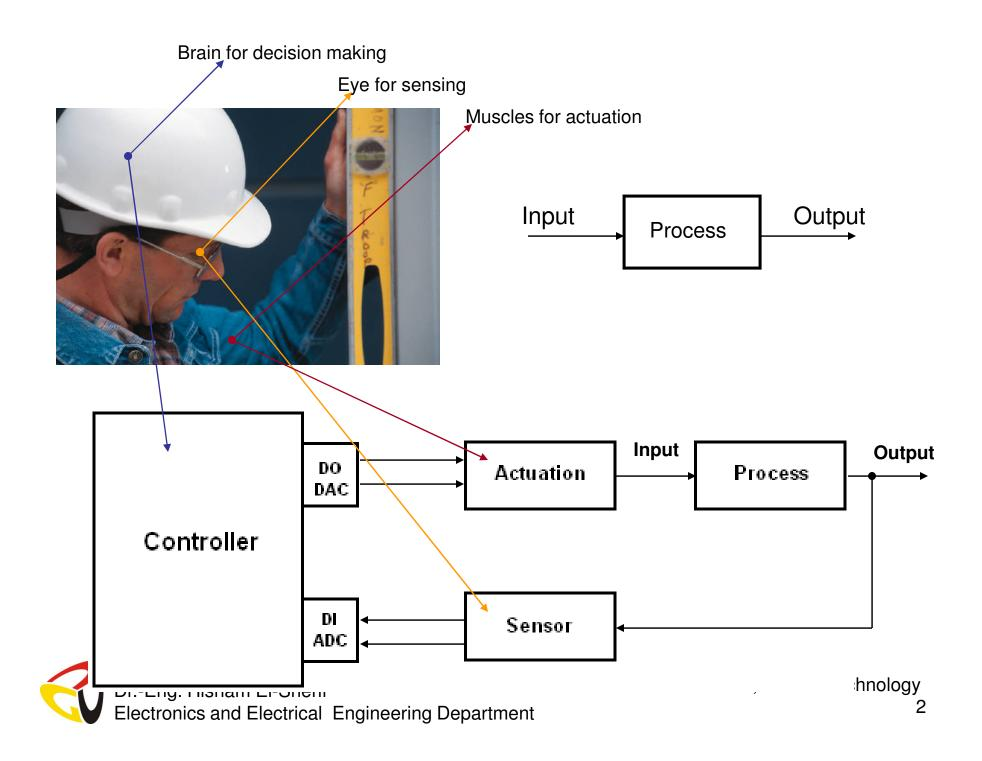
Every computer controlled system has these four basic functional blocks:-
