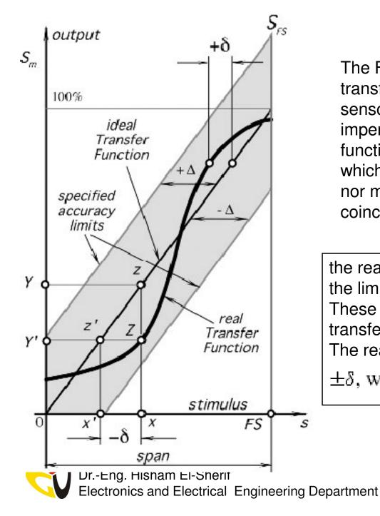
The Figure shows an ideal or theoretical transfer function. In the real world, any sensor performs with some kind of imperfection. A possible *real* transfer function is represented by a thick line, which generally may be neither linear nor monotonic. A real function rarely coincides with the ideal.
