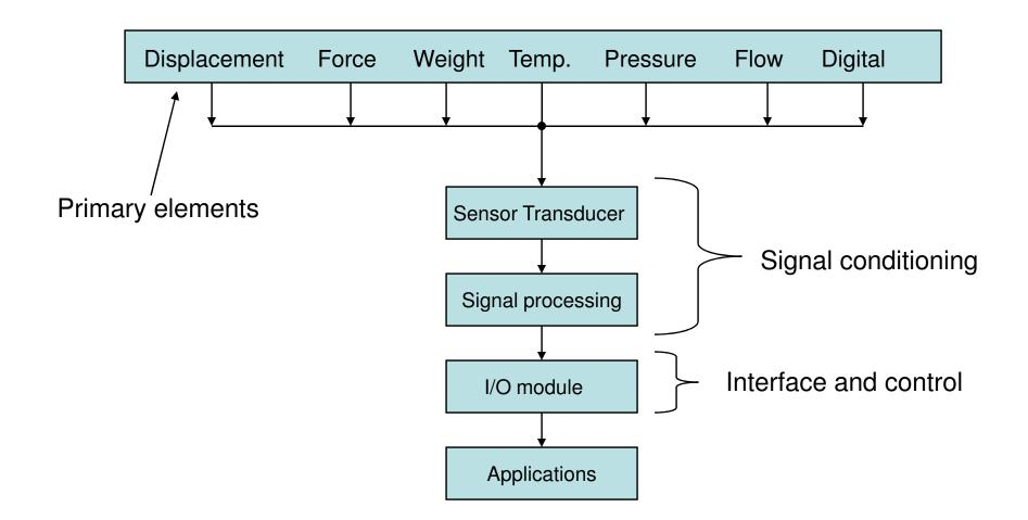
Instrumentation used for general sensing applications
