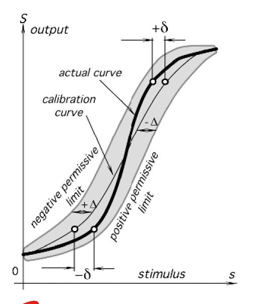
The Figure shows that  $\pm \Delta$  may be more closely follow the real transfer function, meaning better tolerances of the sensor's accuracy. This can be accomplished by a multiple-point calibration. Thus, the specified accuracy limits are established not around the theoretical (ideal) transfer function, but around the calibration curve, which is determined during the actual calibration procedure.
