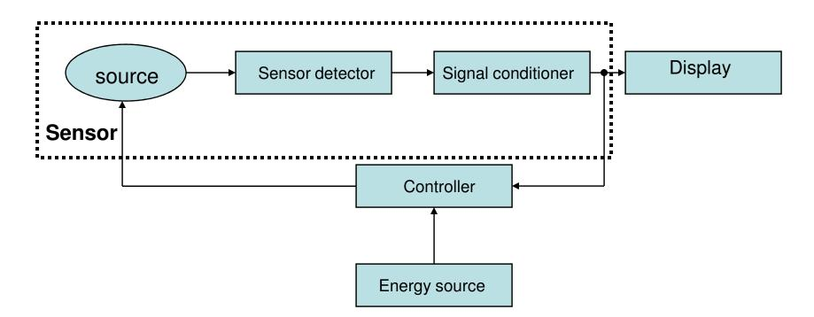
Sensor detector :- to sense the information of interest and convert this information into an acceptable form of signal conditioner.
