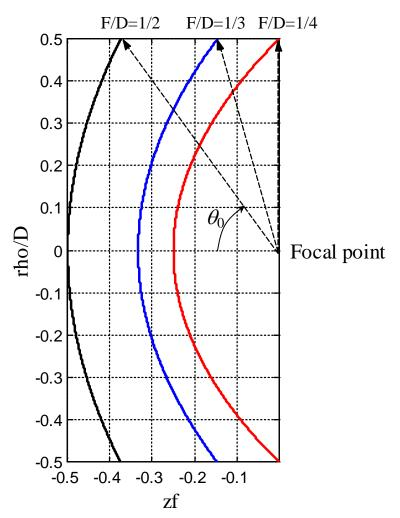
The angle from the feed (focal) point to the reflector's rim is related to F / D as
