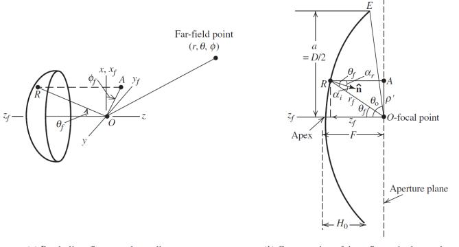
(*a*) Parabolic reflector and coordinate system.
