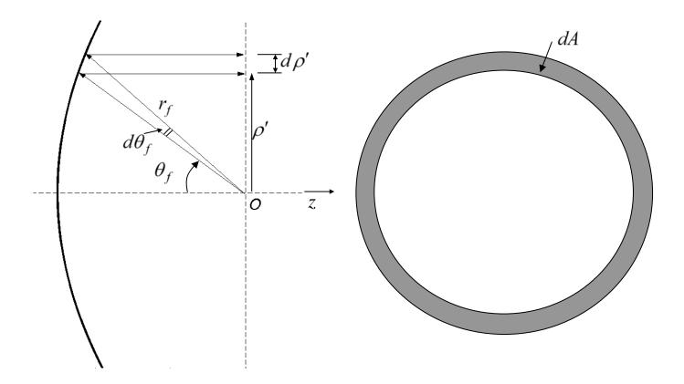
GO assumes that the power density in free space follows straight paths. Applied to the power transmitted by the feed, the power in a conical wedge stays confined within as it progresses along the cone's axis. Consider a conical wedge of solid angle  $d\Omega$  whose cross-section angle is  $d\theta_f$ . It confines power, which after being reflected from the paraboloid, arrives at the aperture plane confined within a cylindrical ring of thickness  $d\rho'$  and area  $dA = 2\pi\rho' d\rho'$ .
