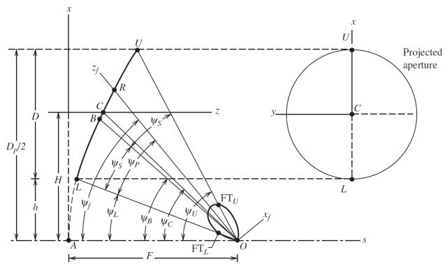
**Figure 9-31** Geometry of the offset parabolic reflector of diameter D and focal length F. The axis of symmetry s bisects the parent parabolic curve of diameter  $D_p$ . Note that the axisymmetric case occurs when H = 0.
