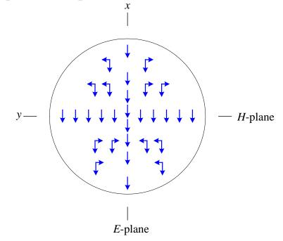
We also note that cross-polarization decreases as the ratio F/D increases. This follows from (19.4), which gives the largest feed angle  $(\theta_f)_{\text{max}} = \theta_0$ . As F/D increases,  $\theta_0$  decreases, which makes the cross-polarization term in (19.39) smaller. Unfortunately, large F/D ratios are not very practical.
