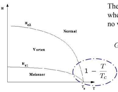
The *lower critical field*  $H_{C1}$  is the phase boundary where equilibrium between having one vortex and no vortex in the superconducting state.
