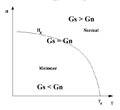
At zero magnetic field in the superconducting phase
