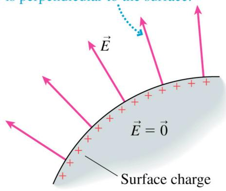
The electric field inside the conductor is zero.
