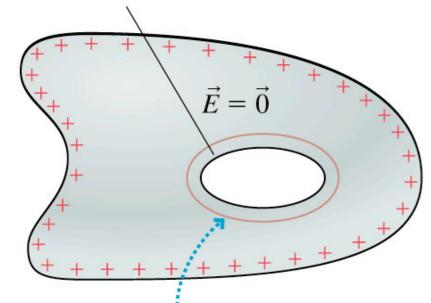
The flux through the Gaussian surface is zero. There's no net charge inside, hence no charge on this interior surface. Parallel-plate capacitor
