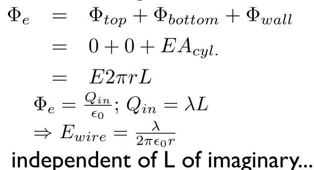
cylinder encloses only part of wire's charge: outside does not contribute to flux, but essential to cylindrical symmetry (easy
