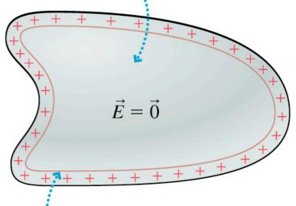
The flux through the Gaussian surface is zero. There's no net charge inside the conductor. Hence all the excess charge is on the surface.
