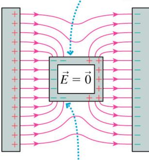
The electric field is perpendicular to all conducting surfaces.
