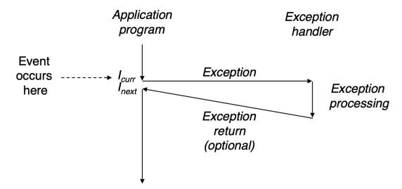
A change in the processor's state (an event) triggers an abrupt control transfer (an exception) from the program to an exception handler. After it finishes processing, the handler either returns control to the interrupted program (to either the same instruction or the next one) or aborts.
