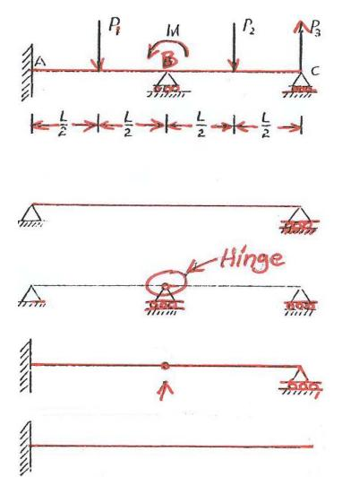
If a structure is statically indeterminate to more than one degree, the approach used in the preceeding example must be further organized and more generalized notation is introduced.
