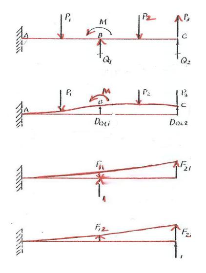
The redundants chosen are at *B* and *C*. The redundant reactions are designated  $Q_1$  and  $Q_2$ .
