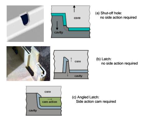
Figure 19. Examples of molds with complex parting lines, and a multi-part mold
