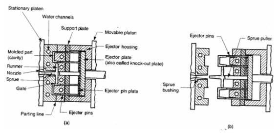
Figure 12(a). A two-plate mold
