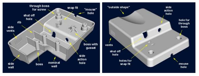
Figure 18. Examples of different shape features in typical injection molded parts [source: www.idsa-mp.org]
