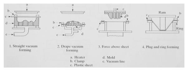
Figure 3. Schematic of thermoforming processes [source: Kalpakjian and Schmid]
