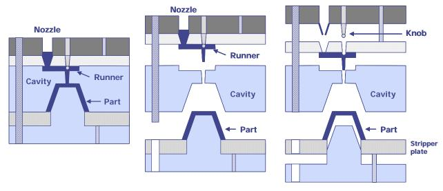
Figure 17. The mold in operation
