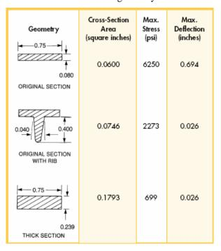
Figure 20. Comparison of breaking stress under bending moments on bars of different cross-section geometry
