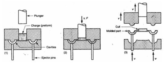
FIGURE 8. Schematic of Transfer Molding
