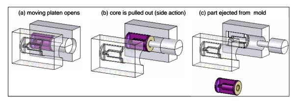
Figure 13. Injection molding a part with side action using core
