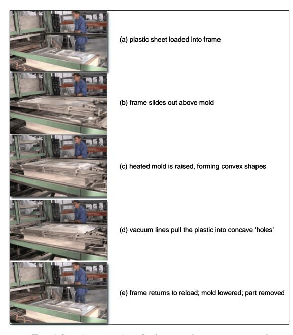
Figure 4. Stages in a vacuum thermoforming process [source: www.ymlf.com.hk]
