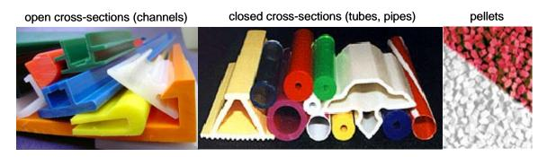
Figure 2. Parts made by extrusion [sources: websites of keltrol.com, seilerpc.com]
