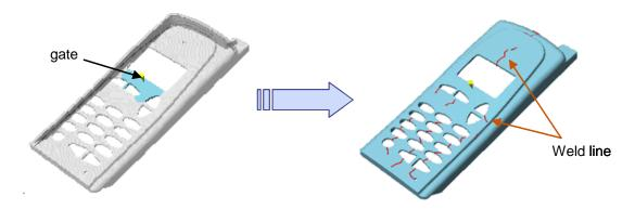
Figure 24. Due to location of the gate and the geometry of the cavity, the front of the flowing plastic meets along several lines, called weld lines
