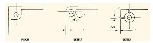
Figure 23. Example of improving design for injection molded parts
