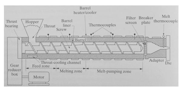
Figure 1. Extrusion machine schematic [source: Kalpakjian and Schmid]
