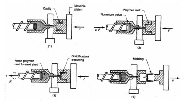
Figure 10. Cycle of operation for injection molding [source: www.offshoresolutions.com]
