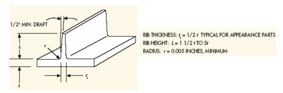
Figure 21. Guidelines for rib dimensions
