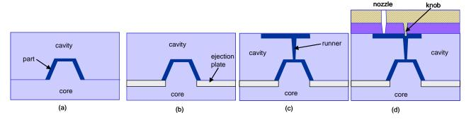
Figure 16. Stages of development of the injection mold
