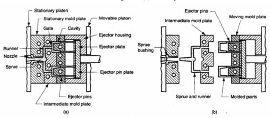
Figure 12(b). A three-plate mold
