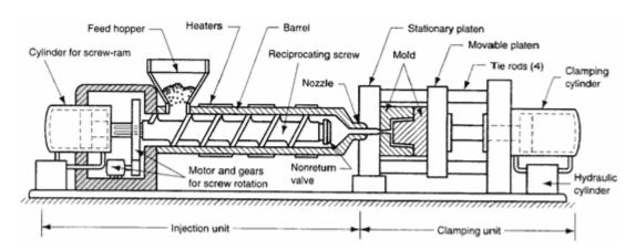
Figure 9. A simple reciprocating screw injection molding machine [source: www.offshoresolutions.com]
