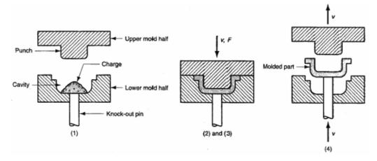
Figure 7. Schematic of Compression Molding
