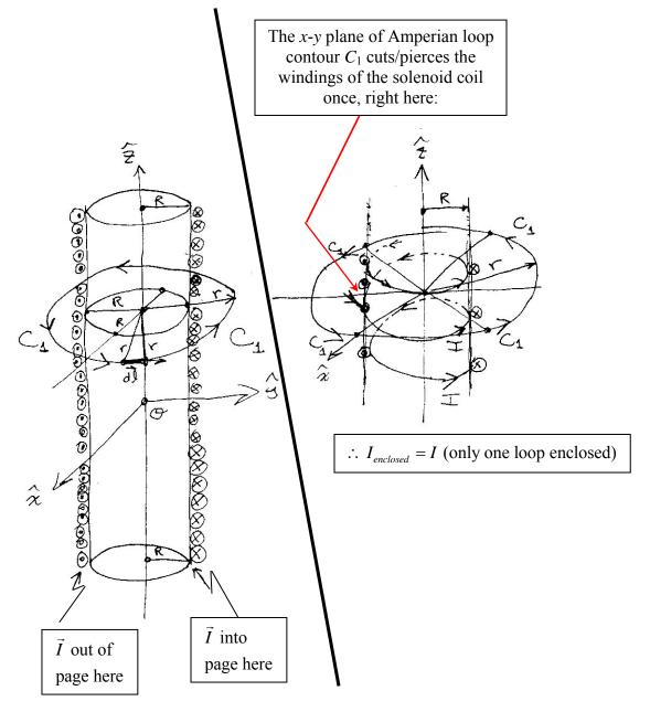
n.b. The finite pitch angle  $\alpha$  associated with the windings of a solenoid coil arises due to winding the coil with wire of finite thickness (e.g. wire radius = *a*). For  $a \ll R$ , then:  $\tan \alpha \approx \alpha = 2a/R$ .
