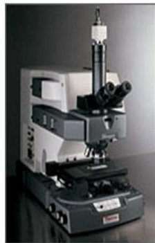
Figure 1 The configuration of a Fourier transform infrared (FTIR) spectroscopic imaging device consists of an interferometer coupled to a microscope and IR-sensitive focal plane array detector. When a conventional, single-element detector is employed ( right ), the microscope is necessarily equipped with apertures and a precision stage. For multichannel detection ( left ), no apertures are required.
