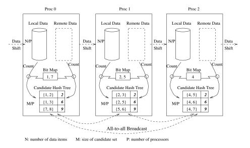
Fig. 6. Intelligent Data Distribution (IDD) Algorithm
