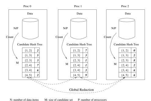
Fig. 4. Count Distribution (CD) Algorithm
