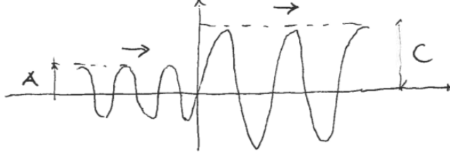
Figure 6.9: Potential step; case E > V_0 . Incoming and transmitted wavefunctions.
