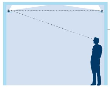
For coves more than 9 ft (2.7 m) from the floor, find the farthest point from which the cove is visible at a height of 7 ft (2.1 m), and draw a line from that point through the top edge of the cove fascia to the back of the cove.
