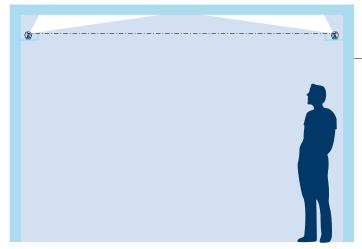
For coves less than 9 ft (2.7 m) from the floor, determine the line of sight by drawing a horizontal line from the top edge of the cove fascia to the back of the cove.
