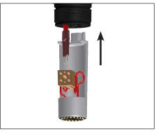
**18.** Connect the bus wires of the trace heater to the terminal block.
