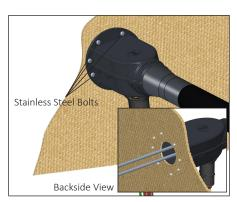
**13.** Secure FAK-1 to bulkhead/wall using (8) eight stainless steel bolts. Note: stainless steel bolts, washers, and nuts provided by others. Recommended bolt size is 8-32.
