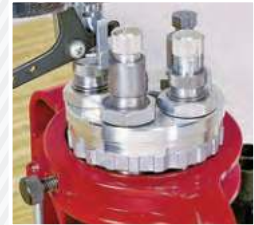
Precision 5-Hole Turret with 20 locking lugs takes just seconds to change. 90079 16.00
