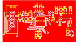
Figure 23: Power Evaluation PCB Top
