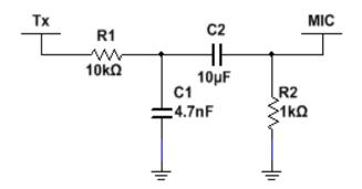
Figure 11: Transmit Circuit
