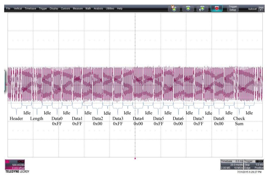
Figure 17: Smartphone Transmission
