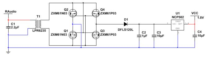
Figure 2: Power Circuit
