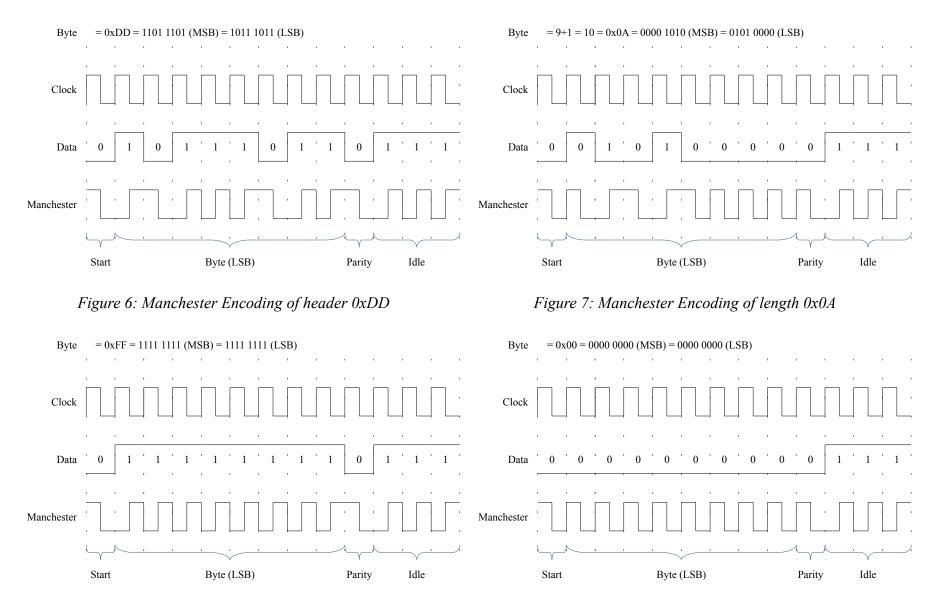
Figure 8: Manchester Encoding of data 0xFF
