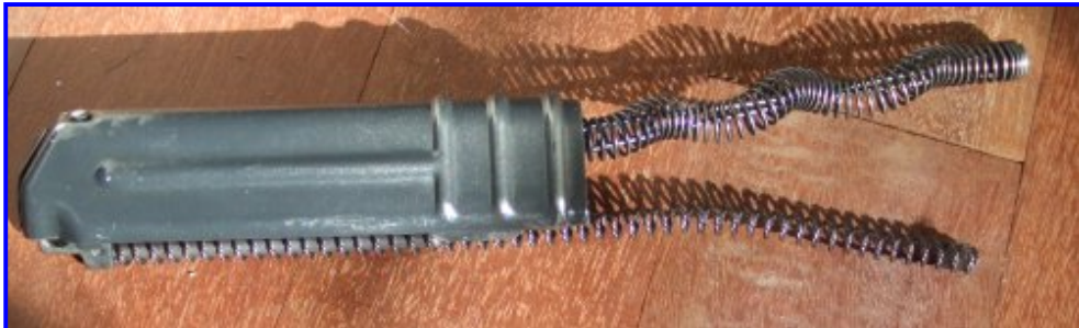
Left: VZ-58 receiver cover, with bolt and striker springs, retained by push out pin with detent stops in the receiver.
