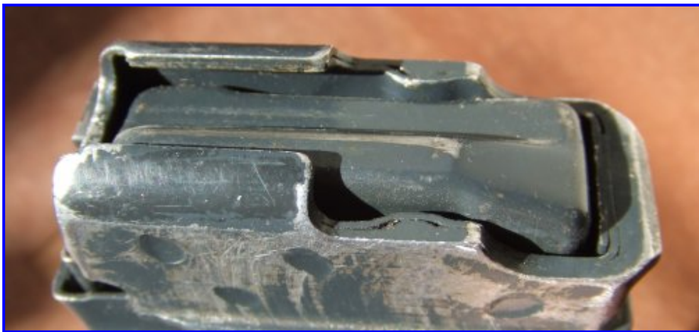
Left: End view of VZ-58 magazine, notice exposed floorplate on rear edge that engages the bolt holdopen.
