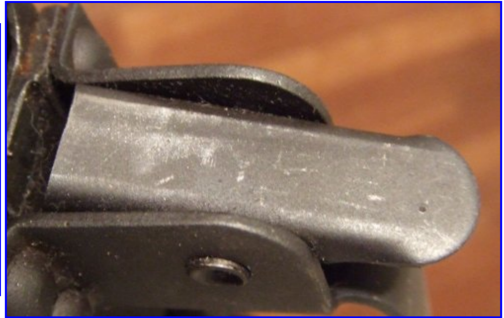
Right: AK-47 paddle type magazine latch centered.
