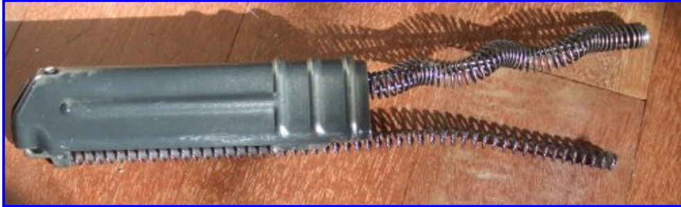
Left: VZ-58 receiver cover, with bolt and striker springs, retained by push out pin with detent stops in the receiver.
