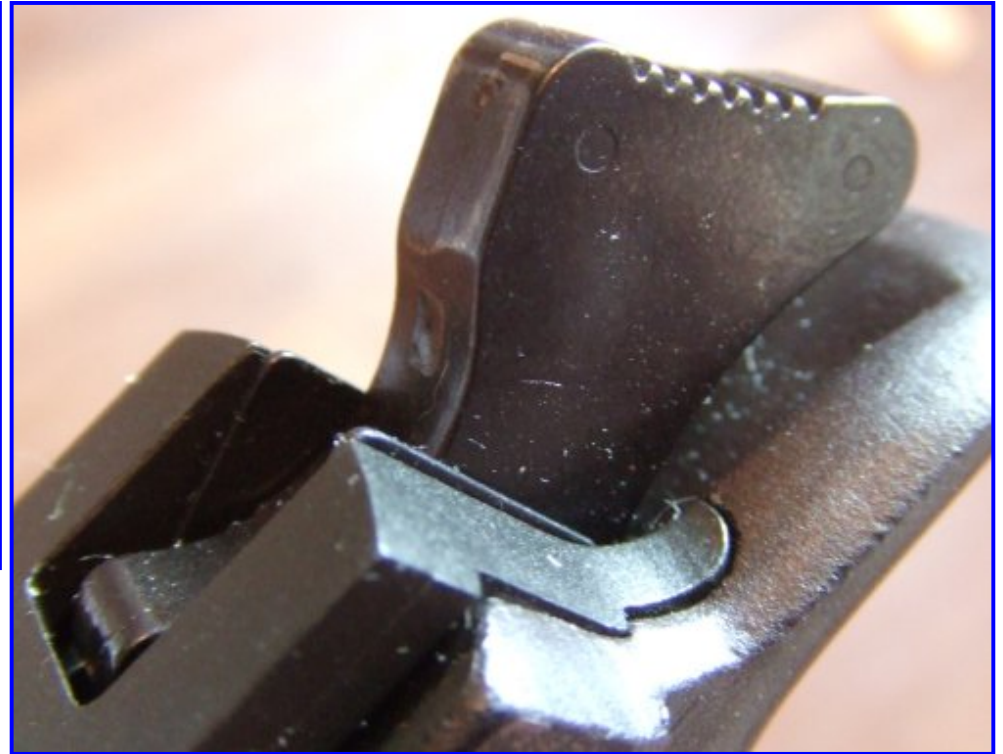
Right: Desert Eagle hammer cocked inside frame.
