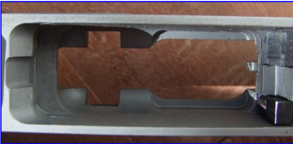
Left: VZ-58 magazine well milled into receiver.
