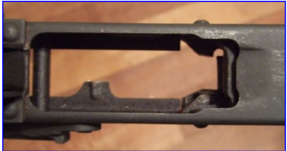
Right: AK-47 magazine well with stamping in receiver to constrict it and hold the magazine tightly
