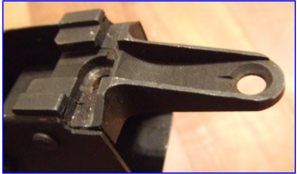
Right: AK-47 rear trunion with tang that end of stock slides into and through which screws are inserted.
