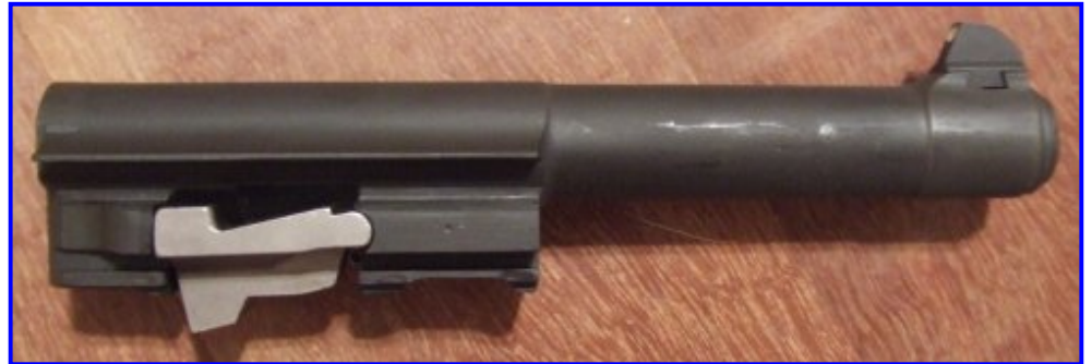
Right: P-38 barrel assembly removed, lug in unlocked position.
