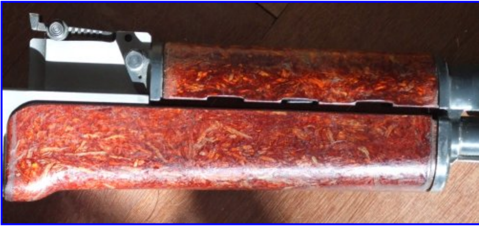
Left: VZ-58 top handguard retained by detent secured pin at its rear.
