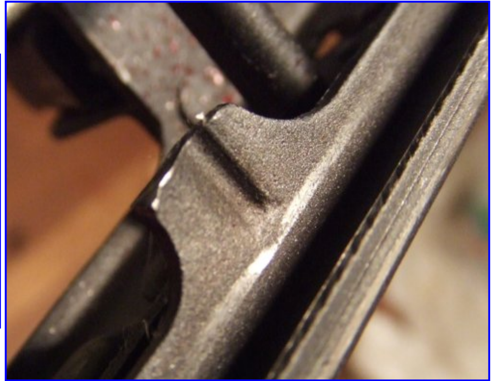
Right: AK-47 ejector is integral to the lower rail that the bolt rides on.
