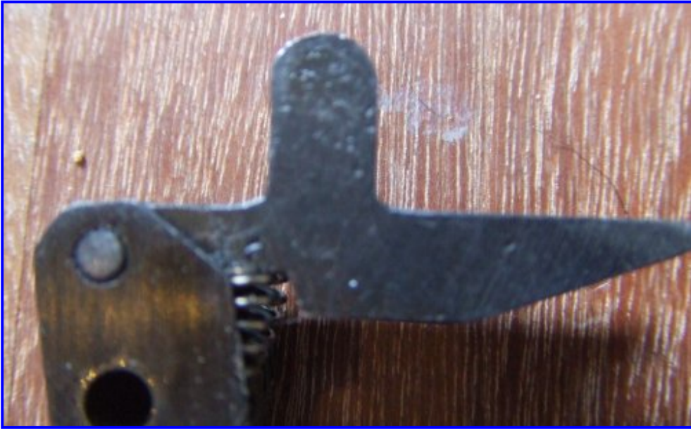
Image: disconnector protrusion on semi-auto trigger arm.
