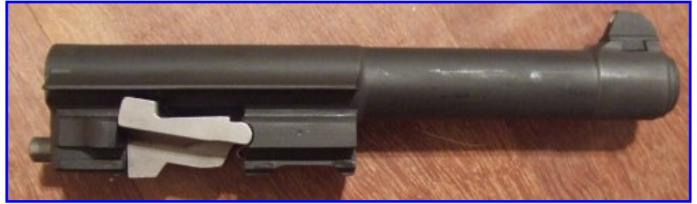
Right: P-38 barrel assembly removed, lug in locked position.
