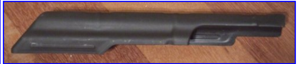
Right: AK-47 receiver cover retained by protrusion on protrusion of the recoil spring assembly that slides into the rear trunion.
