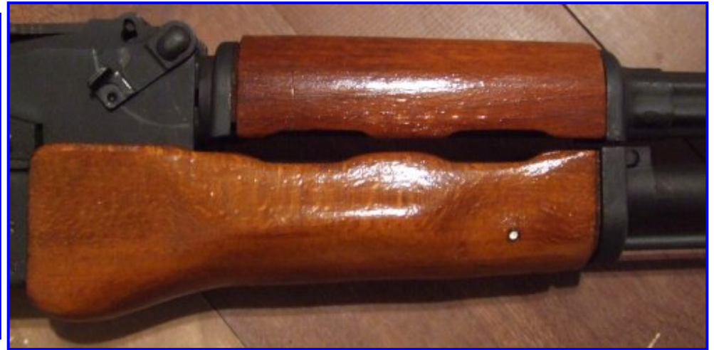
Right: AK-47 top handguard retained by lever at its rear.
