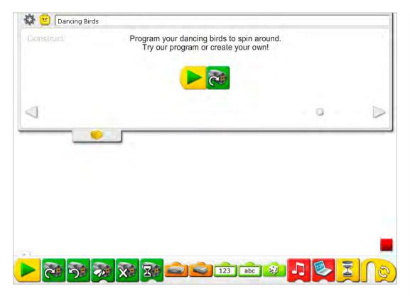
The dancing birds program uses the Start and the Motor This Way Blocks to turn on the motor.
