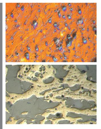
Upper image: Coated and annealed brass sample in LED brightfield-oblique contrast, 500x, Lower image: Plastic composite material in LED brightfield-oblique contrast, 200x. 3D-like image due to oblique illumination.
