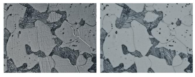
Undereutectoid, ferrit-perlite grain structure LED brightfield-oblique contrast, N Plan 100x Undereutectoid, ferrit-perlite grain structure LED brightfield contrast, N Plan 100x
