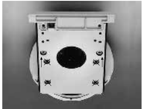
Fig. 26 Objective centering nosepiece*: Screws for tube slit/IC objective prism turret changeover. The other screws must not be loosened under any circumstances.
