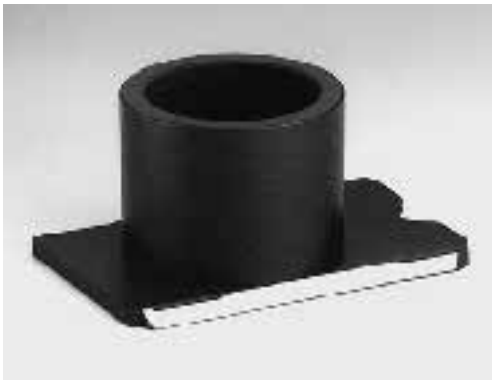
Fig. 64 Light trap for fluorescence microscopy (instead of the condenser). Instead of the light trap, a dark metal or plastic strip can be used, which is inserted between the upper and lower part of the x/y stage under the specimen.
