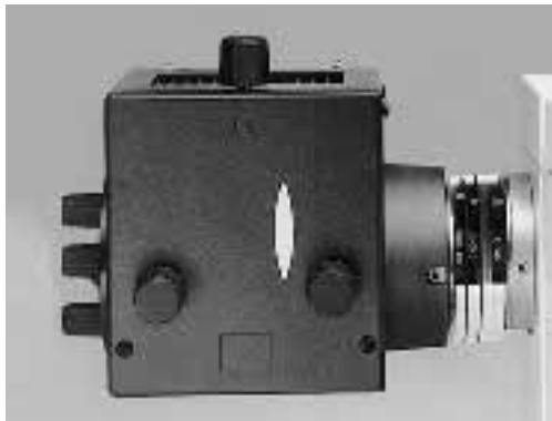
Fig. 9 Filter holder (intermediate unit), with lamphousing for max. 4 filters, dia. 50 mm (when lamphousing 106 is used, only 1 thick or 2 thin filters can be inserted)
