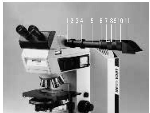
Fig. 67 Macro device on HC FSA 25 PE tube 1 Tube flange, 2 Coupling ring, 3 Reflection optics, 4 Coupling ring, 5 Macro adapter, 6 Screw ring, 7 Zoom setting ring 1 : 4, 8 Scale of zoom factor, 9 Scale of magnification factor of the working distance, 10 Scale of object distance from the bottom edge of the mirror housing, 11 Mirror housing
