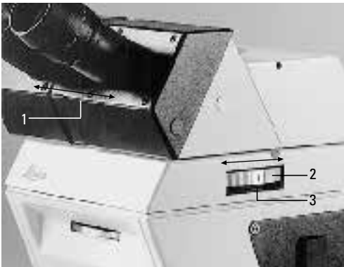
Fig. 50 Tube and tube lens system with Bertrand lens 1 Interpupillary distance setting of the observation tube, 2 Dial for Bertrand lens (B) or tube lens (1x), 3 Focusing of Bertrand lens
