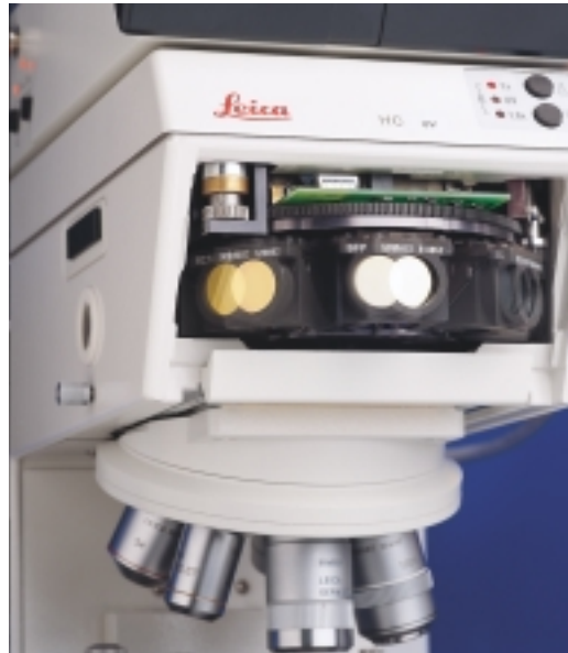
Motorized 8-position fluorescence cube changer with zero pixel shift
