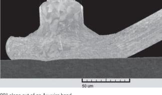
90° slope cut of an Au wire bond
