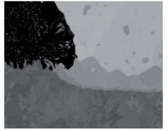
Solder ball after ion beam polishing
