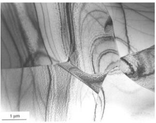
STEM images of a Ti film that has been ion beam milled at an angle of  $6^{\circ}$
