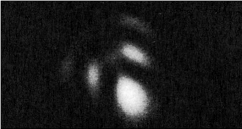
Figure 6 The appearance of a point object due to the presence of coma. Compare with Figure 3.
