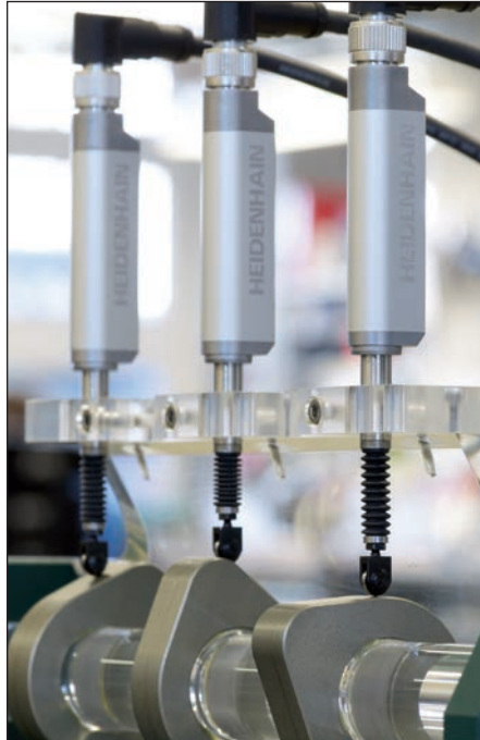
Testing station for flatness inspection
