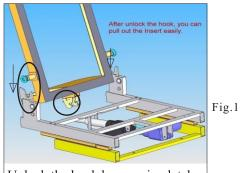
Unlock the hook by pressing latch from recliner piston to pull out insert
