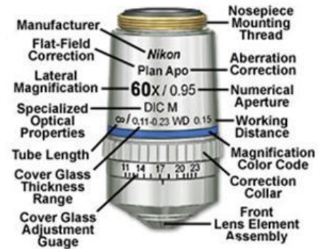
60x Plan Apochromat Objective
