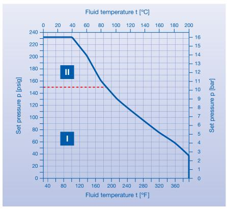
The pressure temperature rating of Type 447 is depending on the PTFEparts in the valve. The diagramm shows the application range of:
