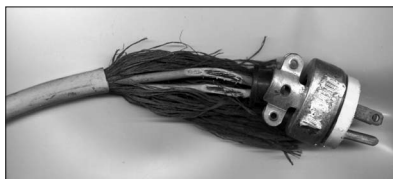
If the plastic insulator of the electric cord breaks, the two wires inside may touch each other. Such contact allows the electrons to flow from one wire to the other instead of first traveling through the appliance. This can heat up the wires enough to cause a fire.
