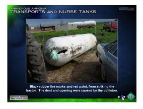
10. The gash, tire marks, and the red paint all were from the collision with the tractor
