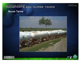
2. Nurse tanks are generally parked together when sitting at a dealer location. This can make it hard to determine which tank is leaking
