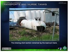
11. The missing shell section remained by the load out risers
