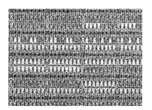
0.35µm Flash in Atmel microcontroller
