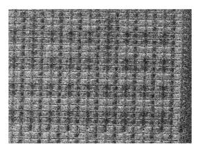
0.35µm Flash in TI microcontroller 15
