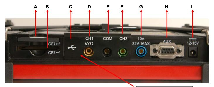
**A** – Compact Flash Slot 1 (CF1) Contains All Operating Software (Do Not Remove) Slide Cover to reveal USB Ports
