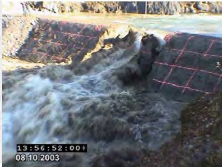
c. Soil block fails and rotates into breach flow (removed completely within 10s)
