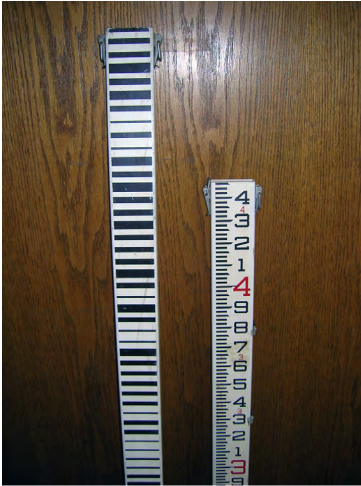
Figure 4. Bar-code leveling rods. A. separated multi-section rod showing the self-reading rod scale on the second side.
