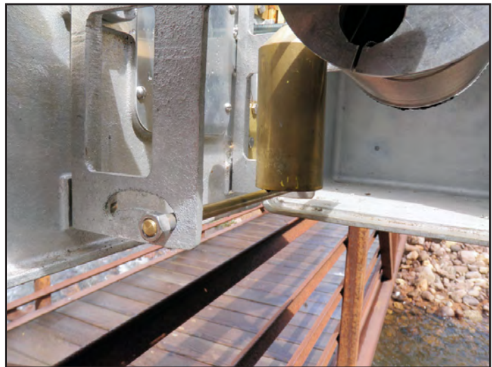
Figure 19. Wire-weight gages mounted on bridges.
