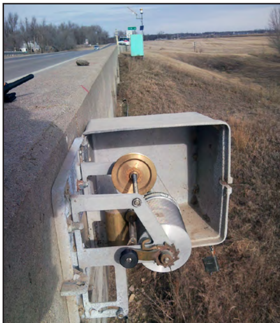
Figure 19. Wire-weight gages mounted on bridges.
