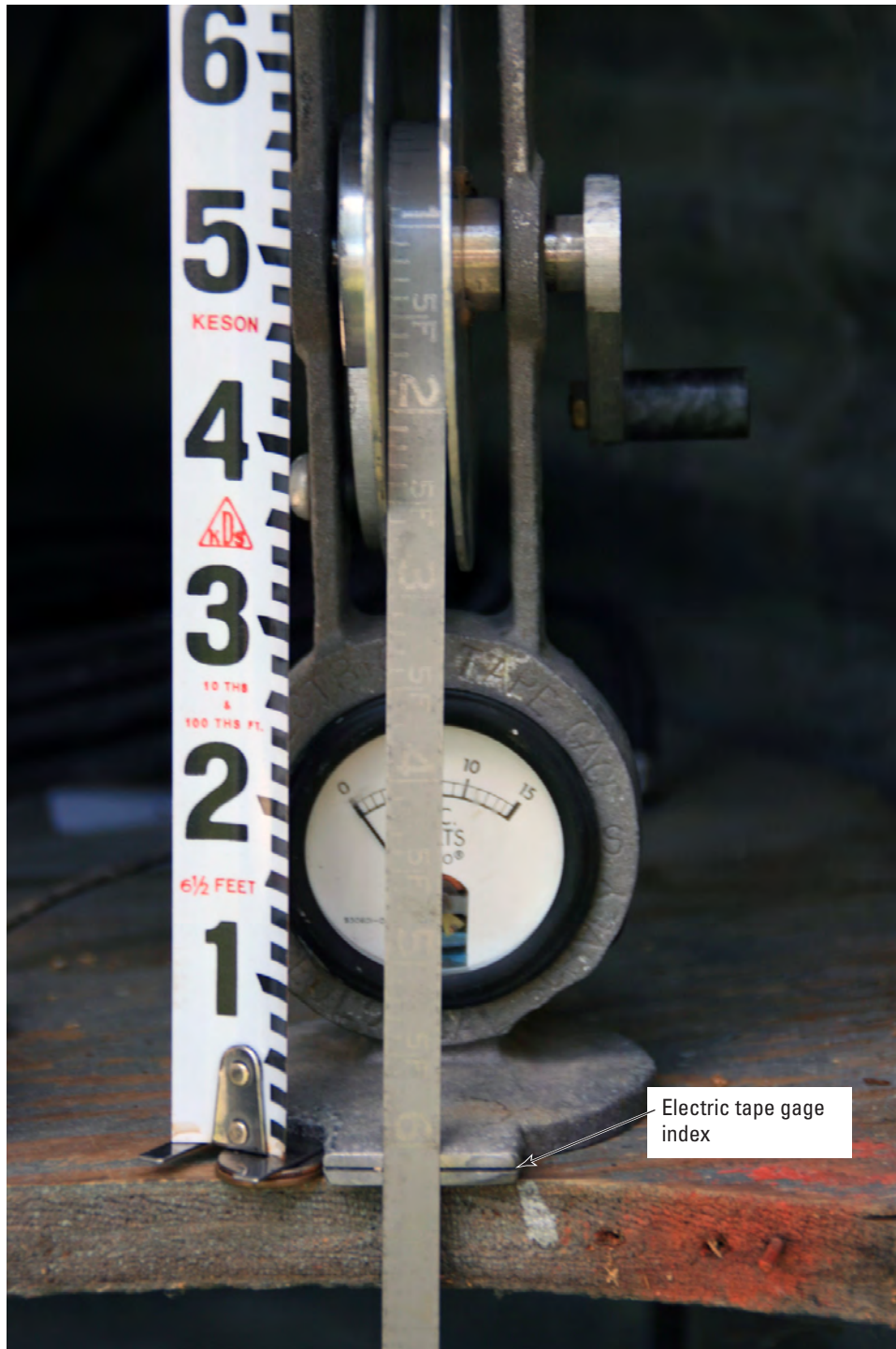
Figure 18. Electric tape gage with a pocket rod held on a stack of coins at the elevation of the index.
