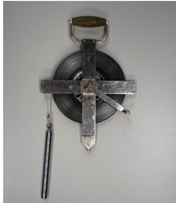
Figure 10. Steel tape with 1 pound of tension.
