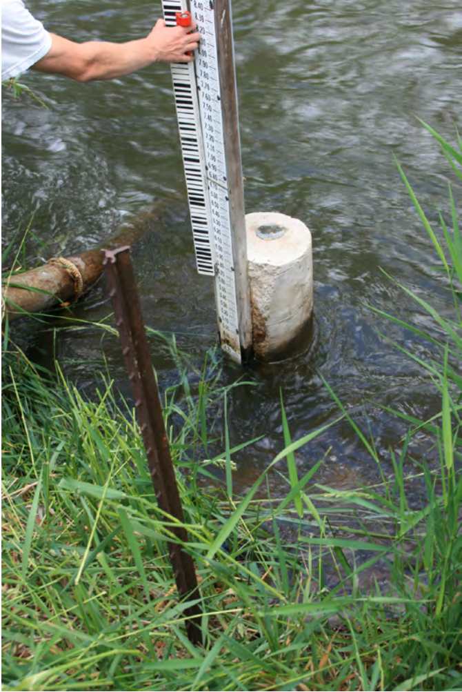
Figure 17. Foresights being taken on staff plates by holding leveling rods on nails driven into backing boards.
