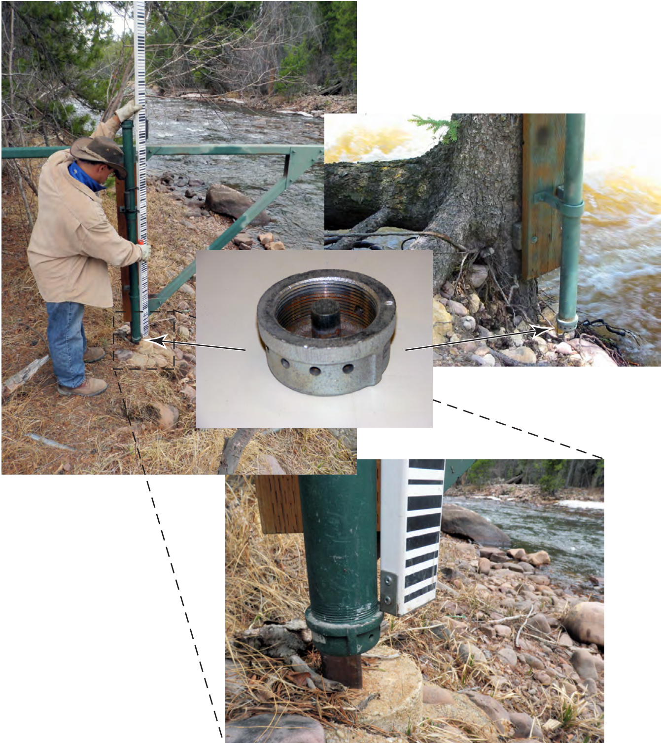
Figure 22. Crest-stage gage where the index is the bottom cap. Inset photograph of the bottom cap showing the internal stud.
