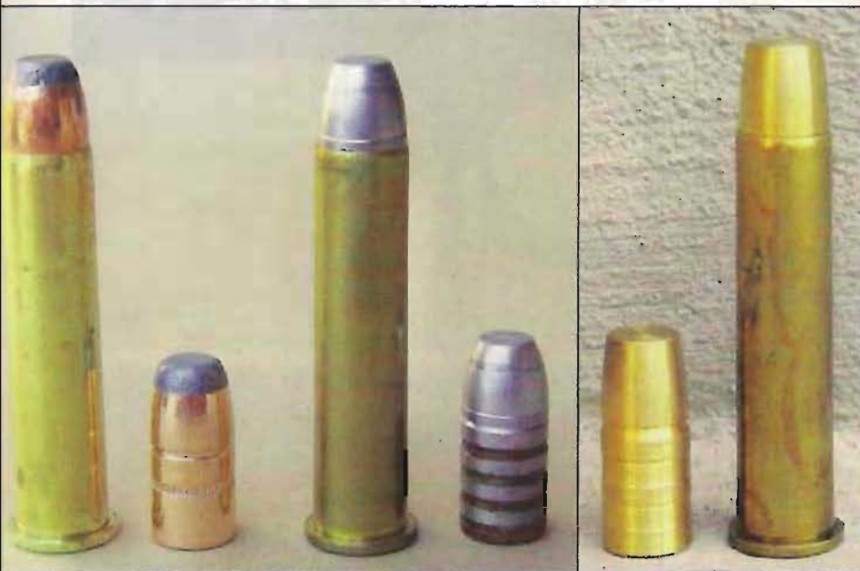
The .45-70 is well-suited to using either jacketed or cast bullets. Belt Mountain offers a superb 400-grain Punch Solid (right) for use in the .45-70, which Brian considers ideal for heavy and dangerous game, including elephant.
