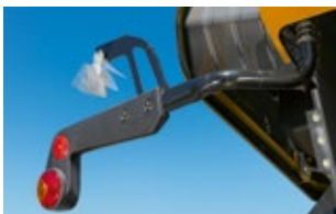
Automatic side-wind/slope compensation sensor.
