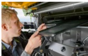
Divided preparation floor can be pulled out towards the front.
