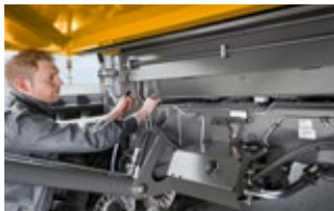
The large rock trap is easy to open from the side and is self-emptying.
