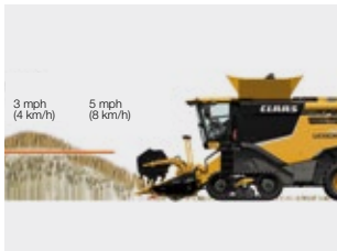
Automatic ground speed control with CEMOS CRUISE PILOT.
