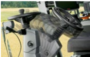
Adjustable steering column.
