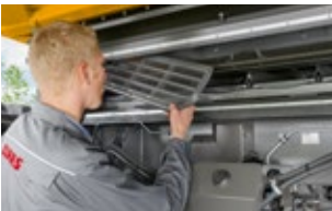
APS pre-concave segments can be changed quickly thanks to the MULTICROP concave.
