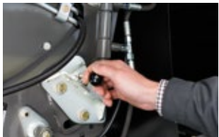
In-cab or manual friction floor and stationary knives adjustment.
