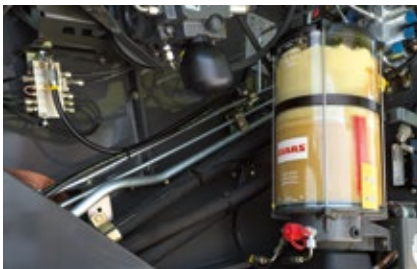
Central lubrication system supplies grease to practically all lubrication service points as required.
