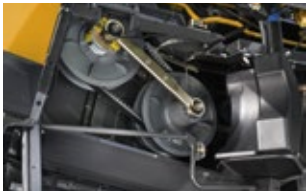
Continuously adjustable variator.
