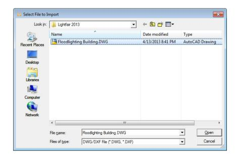
The 2D drawing of the building is imported. The drawing is composed of lines. The lines be converted to solids.
