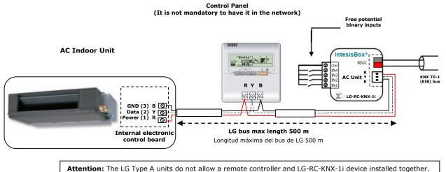
Figure 2.1 LG-RC-KNX-1i connection diagrams
