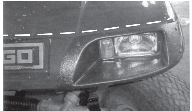
Step 6: Place headlight assembly along body line and install screws.
