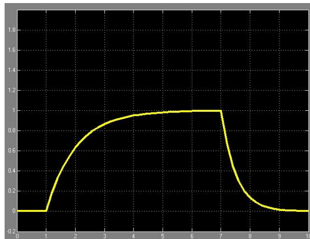
Figure 2-4: Asymmetrical PT1 element step response
