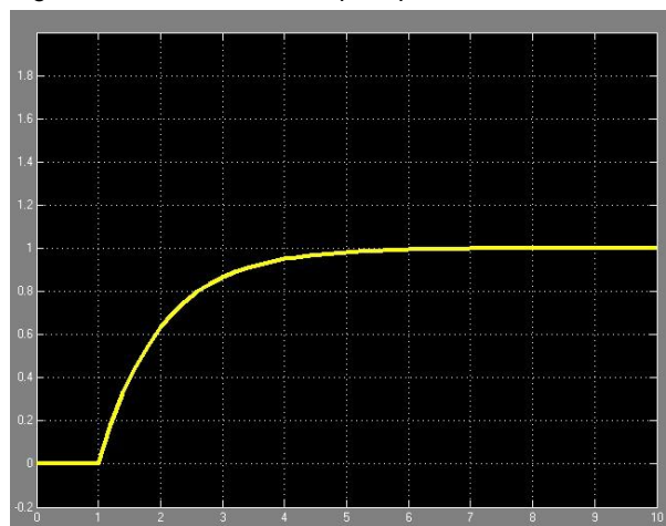
Figure 2-2: PT1 element step response
