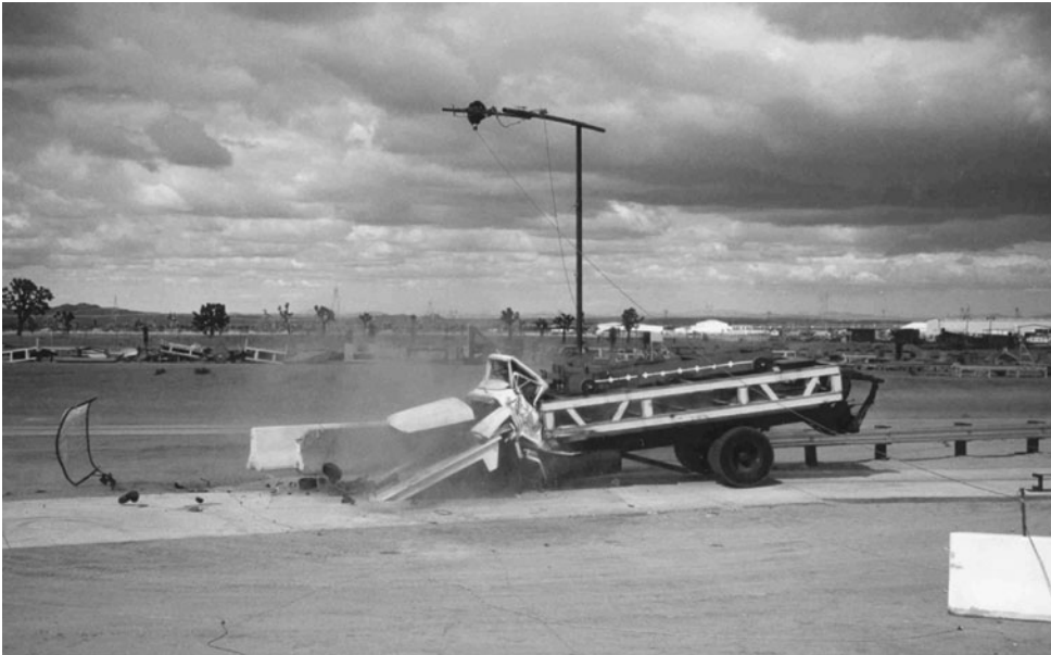
Figure 8-12 Crash gates prevent unwanted vehicles from entering (or leaving) a facility
