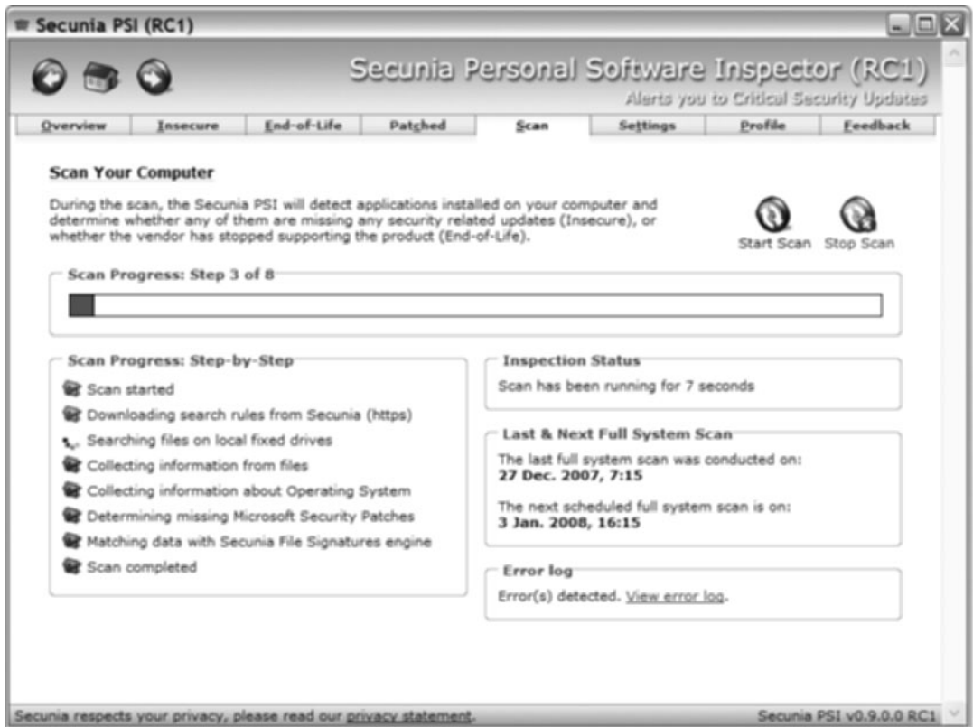
Figure 3-8 Secunia Personal Software Inspector tool scanning for vulnerabilities
