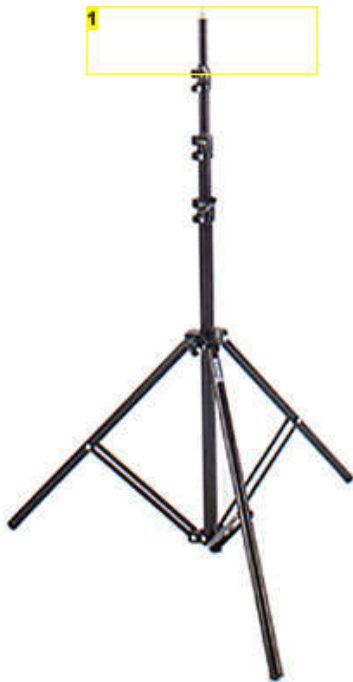
Image Notes 1. this part will fit into the pipe section that's screwed into the flange. You can tape the pipe section and use a bolt as a set screw to make it more rigid.
