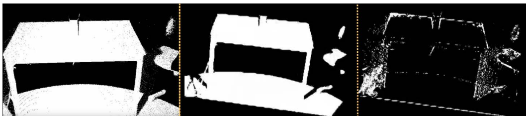
Figure 6.1. An example of noise filtration. Original point cloud in the first picture, processed final point cloud in the second picture and removed points (noise) in the third picture.
