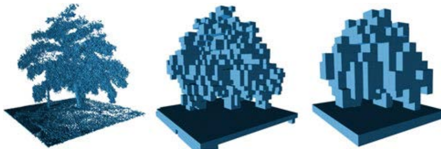
Figure 5.3. Multiple resolutions of the same object. Occupied voxels are displayed in resolution 8 cm, 64 cm and 128 cm. [18]
