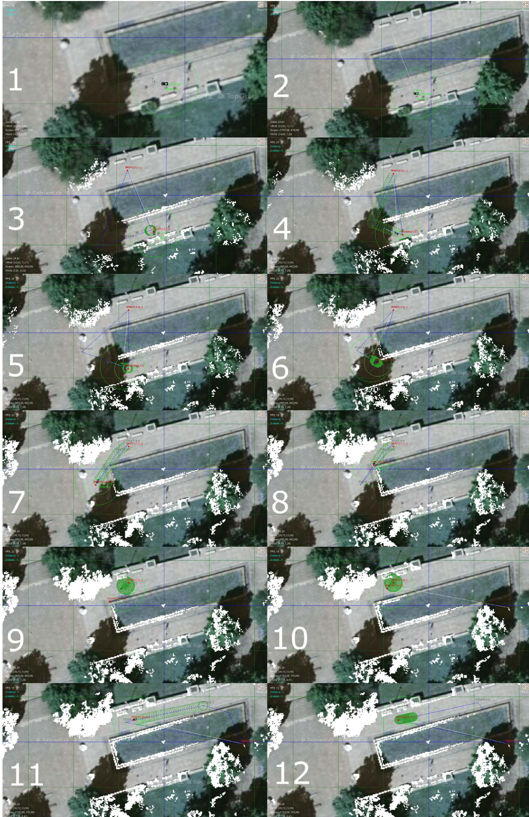
Figure 8.18. Collision avoidance test #2 part 1. Picture number 2 shows the starting and goal position of first target. Pictures 2-9 show how the UGV was moving and the map was incrementally built. In picture 10 another target waypoint was selected and the pictures 11-24 show the progress again. Continuation in Fig. 8.19.
