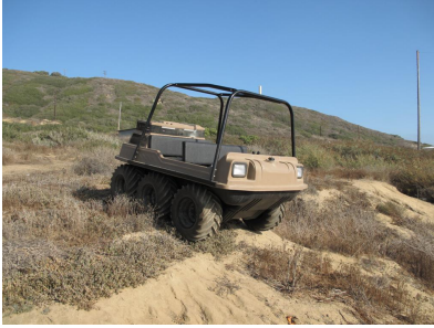
Fig. 2: Max ATV UGV test-bed platform
