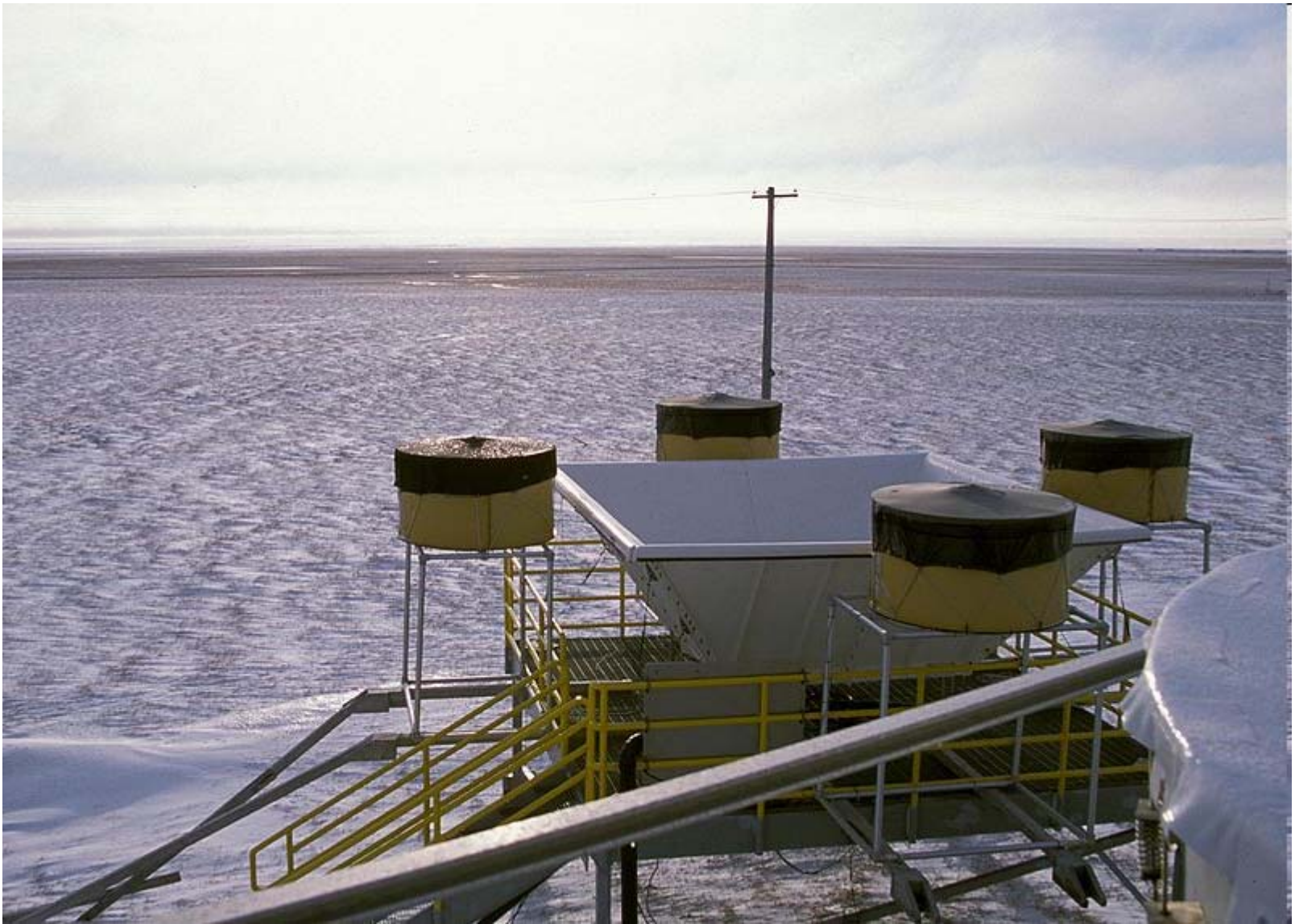
The 915 MHz Radar Wind Profiler (915RWP) and radio acoustic sounding system ( RASS ) at the North Slope of Alaska site in Barrow, Alaska .
