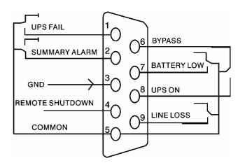
Figure 16.2: DB-9 Interface of AS400 communication protocol
