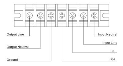
Terminal Block wiring diagram for 6K(L)
