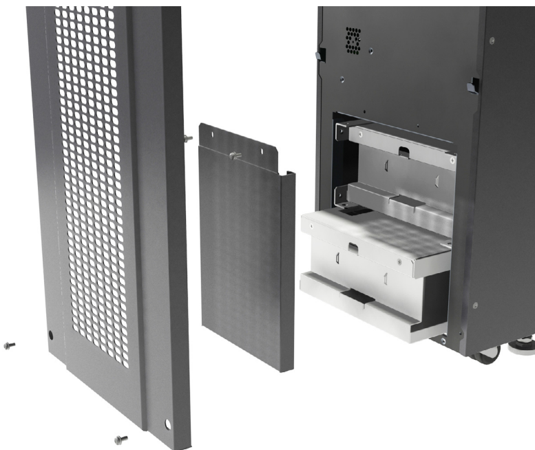
Figure 16 Removing front panel and unlocking battery trays
