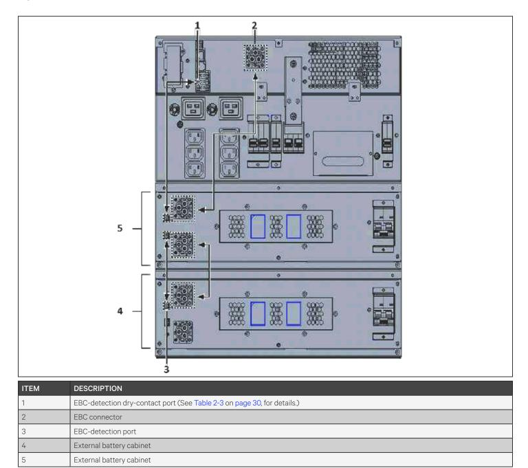
Figure 2-3 EBCs connected to the 8/10 K UPS
