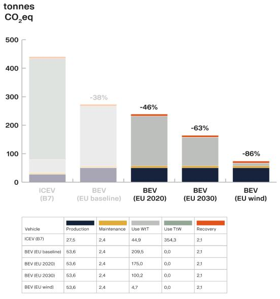
Figure 4. Total life cycle GHG emissions presented as tonnes of  $CO_2eq$  per life cycle phase. The use phase is divided in well-to-tank and tank-to-wheel. Four different grid mix scenarios are used for the use phase electricity.
