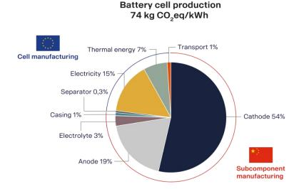
Figure 7. GHG emissions from different steps in battery cell production in % of total impact per kWh installed capacity.
