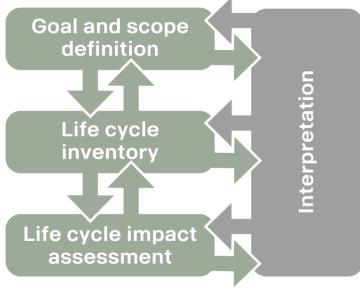
Figure 1. Four stages of the LCA
