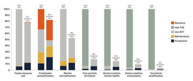
Figure 9. BEV reduction potential for other impact categories. BEV reduction values presented in relation to ICEV emissions.
