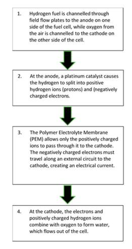
Figure 1. Operating principles of a hydrogen fuel cell [29].
