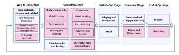
Figure 2. The major stages of process-based PCF estimation on the vehicle cycle of a hydrogen fuel cell car.
