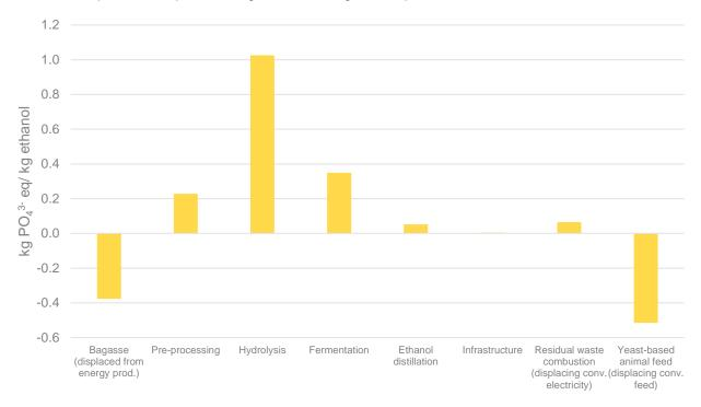
Figure 7 Stage-by-stage breakdown of eutrophication potential from project implementation.
