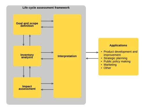
Figure 1 Framework for LCA from ISO 14040.
