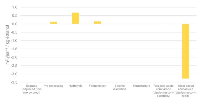
Figure 9 Stage-by-stage breakdown of land occupied from project implementation.
