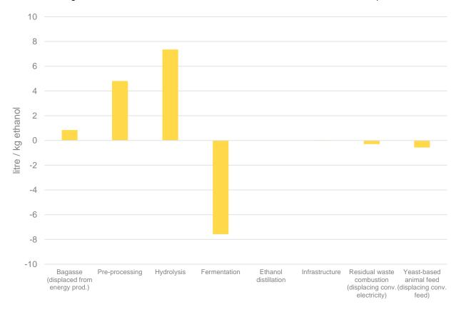
Figure 10 Stage-by-stage breakdown of consumptive water use from project implementation.
