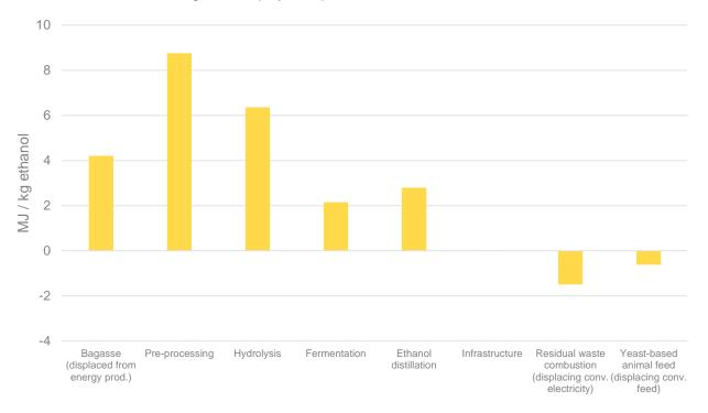
Figure 6 Stage-by-stage breakdown of fossil fuel use from project implementation.
