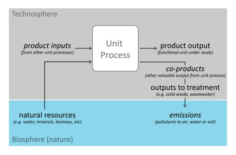
Figure 3 Inputs and outputs of a unit process in LCA.
