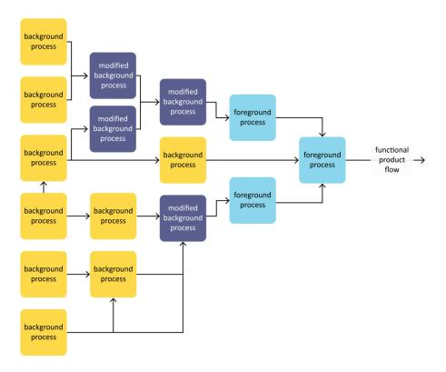
Figure 4 The linking of a unit process in an LCA to produce the functional unit.
