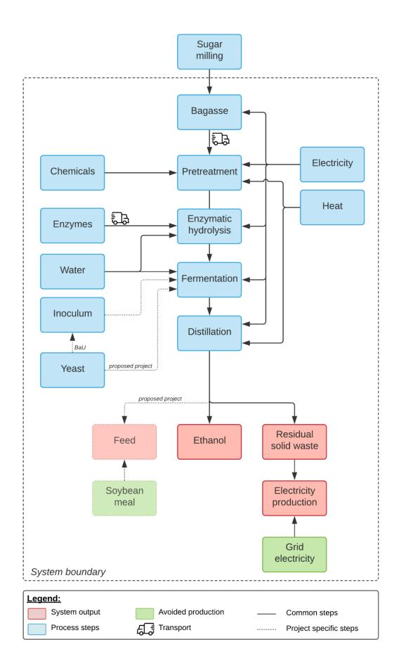
Figure 2 System boundary for the analysis.
